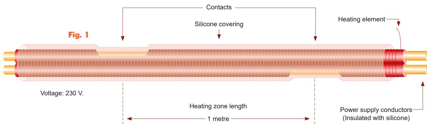
When voltage is applied to the two conductors, the heating conductor receives the same voltage between points of contact: A - B, B - C, C - D, etc. This ensures that the power per linear metre of cable is constant and independent of its length.
